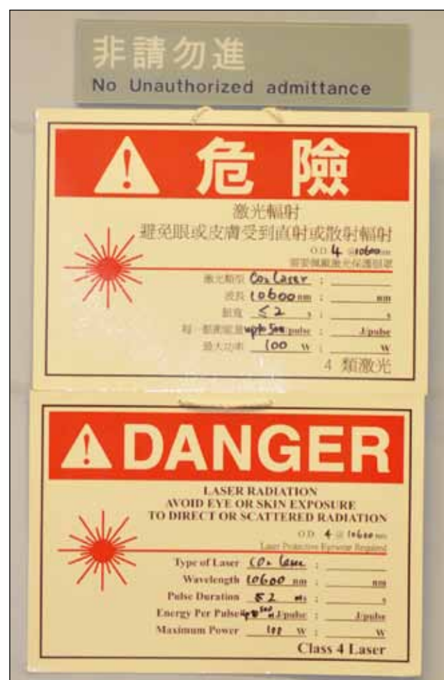
Figure 2. Clearly marked signs for the wavelength of the carbon dioxide laser should be posted on all operating theater doors.
