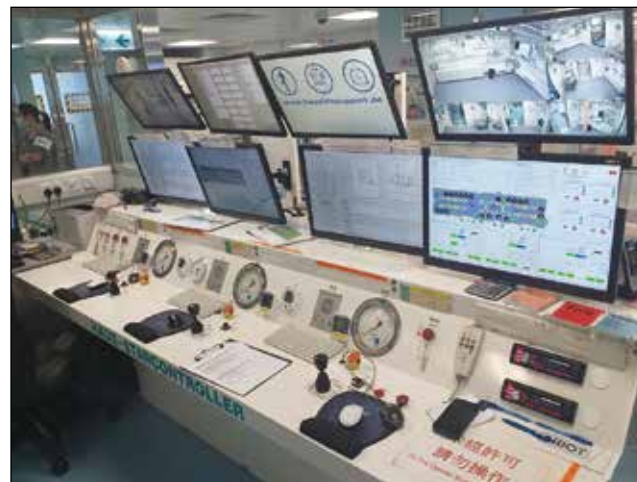
Figure 3. Control station with control panels for opening/closing of doors, working pressures of the chamber, breathing gas (air/oxygen), humidity, temperature, cooling/heating, and fire extinguishing system. Live videos inside the chamber are also displayed.
