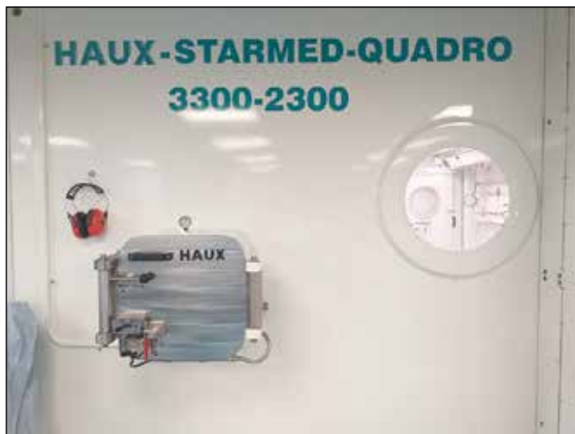
Figure 2. An enabling lock in the hyperbaric oxygen chamber.
