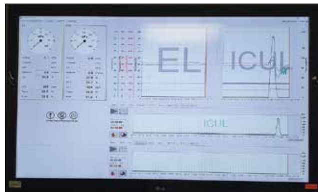
Figure 5. Monitor display of parameters of desired and actual pressure, gradient, oxygen concentration, and temperature.
